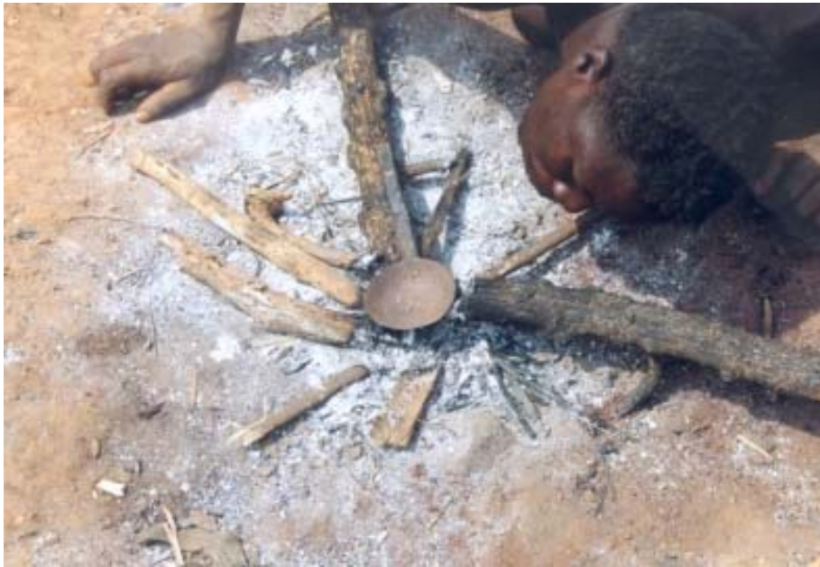
Artisanal Miner burns mercury to amalgamate gold. Source: National Environmental Research Institute (NERI). 2009
